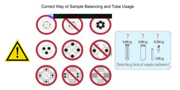
✓ If the number of samples is not in pair, please load the control tubes at each symmetrical position. Otherwise, it results noise and vibration, which eventually damage the instrument
